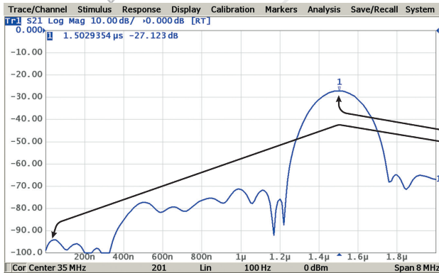
Time domain analysis allows measurements of SAW filters such as the time delay and feedthrough signal suppression.
