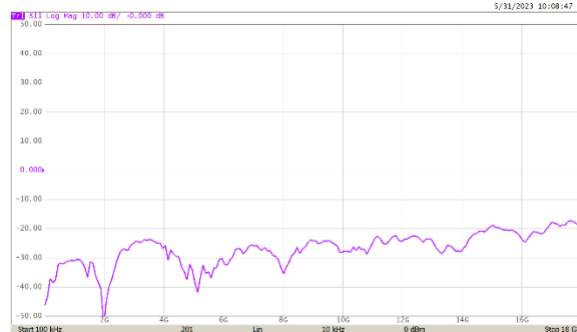
Figure 1- Measurement of a Calibration Load for Test Cable Verification
