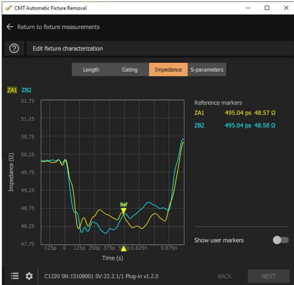
Figure 19 - Fixture Impedance vs Distance
