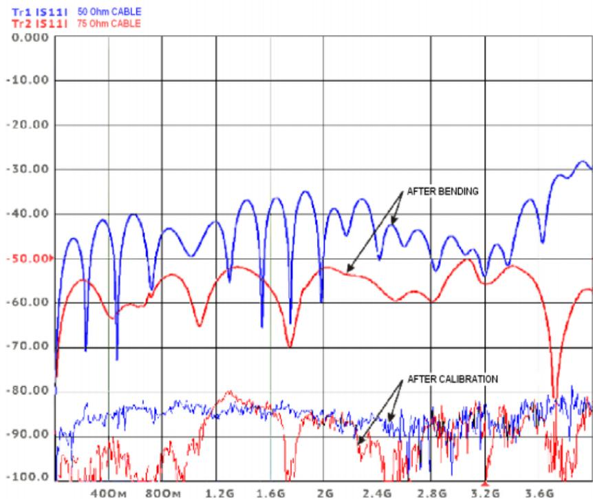
Using CMT Full-Size vector network analyzers with 50Ω test ports, 5.7 dB MLP connected to the VNA test ports, and performing SOLT calibration with a high-quality calibration kit, we can expect the measurement error to be dependent only on the quality of the calibration kit, keeping impact of the 50Ω to 75Ω adapter to a minimum.
