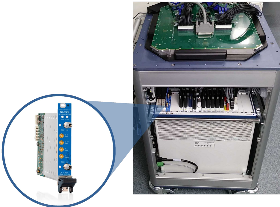
Figure 2 NI STS ATE tester, side panel removed to show CMT S5090 installed inside, SMA cables to loadboard bottom side
