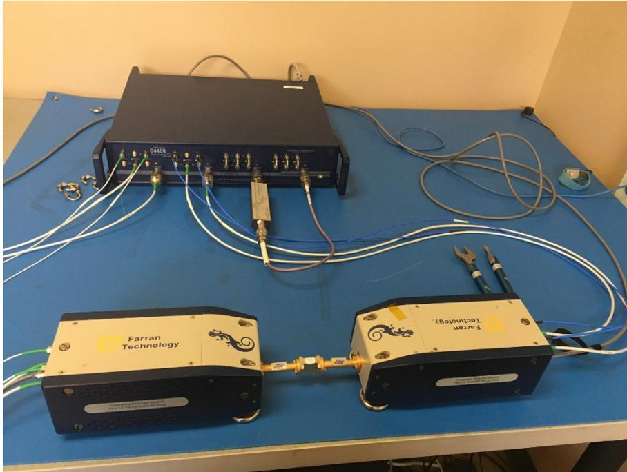
Figure 1: FEV-12 extenders are shown connected to ports 1 & 2, while ports 3 & 4 are connected to the 500 MHz bandpass filter
