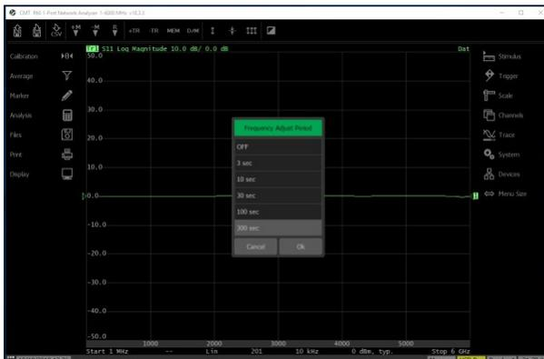
Fig. 2 Assign frequency correction period
