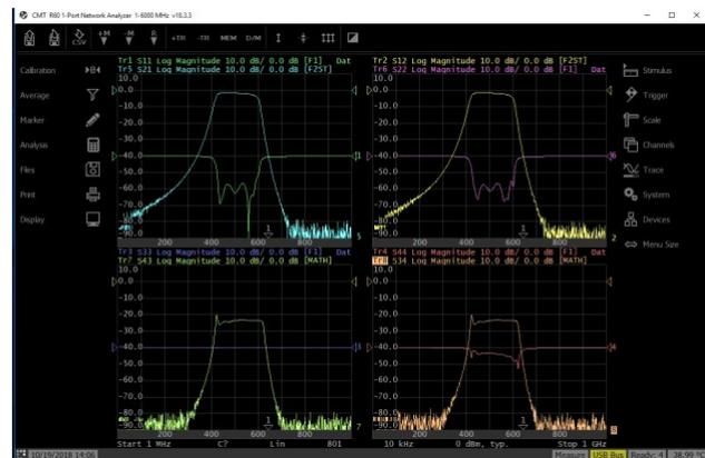
Similarly, one could make measurements of antenna arrays and be able to quickly evaluate the VSWR of each antenna and its isolation to all other antennas in the system. Limit lines and limit tests could be added for fast production test.
