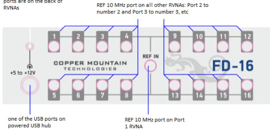
Fig. 6 FD-16 module connection diagram
