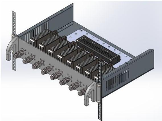
Each 2RU rack shelf can house up to eight 1-Port VNAs. Reflectometer models are available with frequency ranges of 1 MHz to 6 GHz (R60), 85 MHz to 14 GHz (R140) and 1 MHz to 18 GHz (R180). The shelves can only be populated with one model of VNA. It isn't possible to mix them at this time. A powered hub is used to aggregate the separate units to a single USB connection with the host computer and to supply the needed power to the VNAs.
