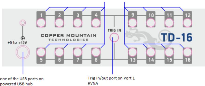
Fig. 4 TD-16 module connection diagram
