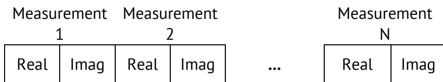
Figure 4. Array of complex measurements
