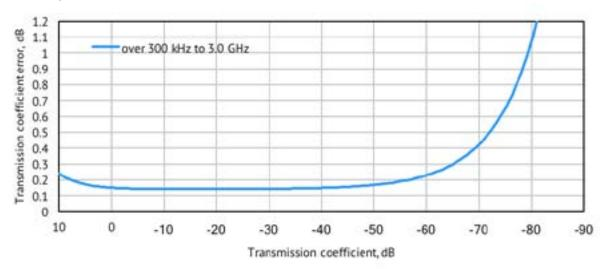
Specifications are based on matched DUT, and IF bandwidth of 10 Hz
