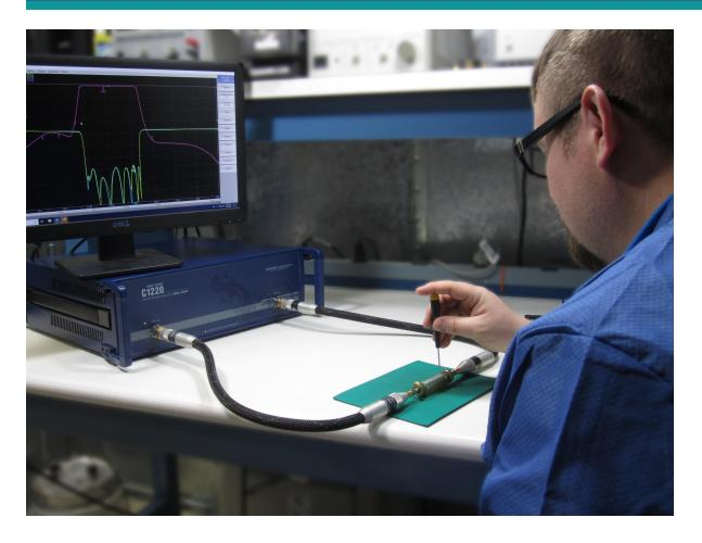
The ability to set pass/fail parameters was helpful for the quality control process and enables Praxsym to quickly teach new employees how to tune filters.
