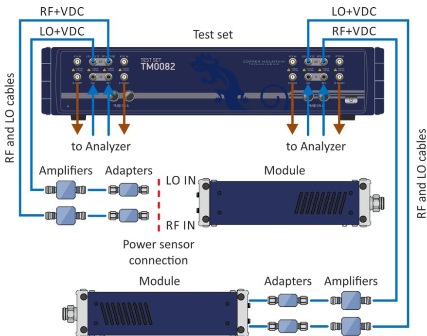
**Figure 4.9** Connection of RF and LO cables, external amplifiers and adapters (do not connect IF cables; no need to connect the modules to power supply)
