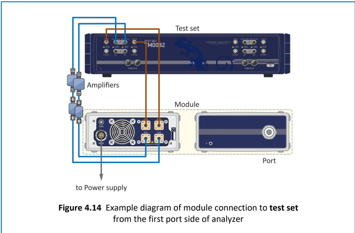
**Figure 4.14** Example diagram of module connection to test set from the first port side of analyzer
