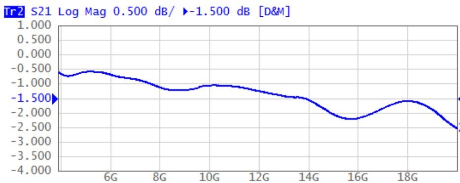
**Figure 2.6** Typical transmission coefficient (insertion loss)
