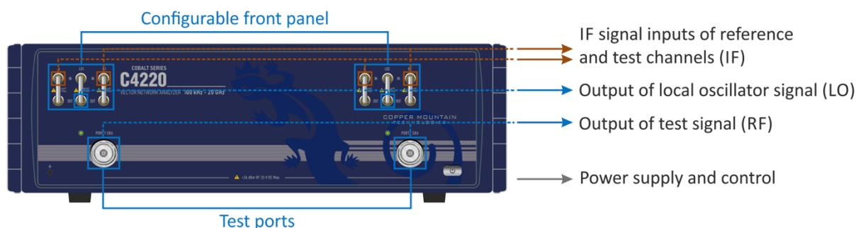
**Figure 1.1** Vector network analyzer. RF measurement module.
