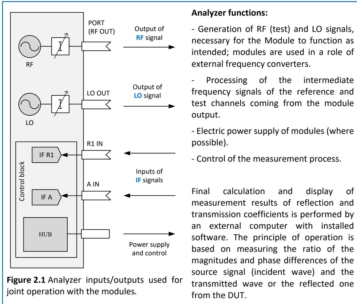
**Figure 2.1** Analyzer inputs/outputs used for joint operation with the modules.
