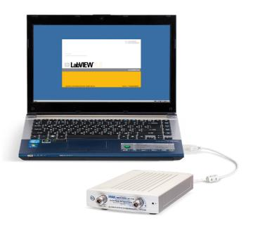
IVI driver can operate without the presence of an actual instrument by using the simulation mode of the VNA software.
