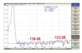
Typical dynamic range of 138 dB is achieved from 1 MHz to 6.5 GHz (at 10 Hz IF bandwidth). Seen here is the maximum dynamic range achieved when using IFBW 1 Hz and an output power level of 5 dBm.
