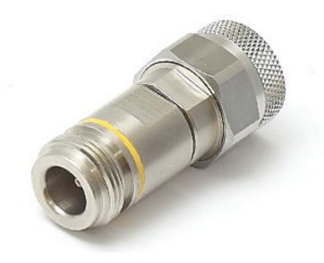
NOTE: The center conductors on 75  $\Omega$  N connectors are smaller than the 50  $\Omega$  versions, and mating a 50  $\Omega$  male with a 75  $\Omega$  female will destroy the female contact, while mating a 75  $\Omega$  male with a 50  $\Omega$  female will result in a poor electrical connection.
