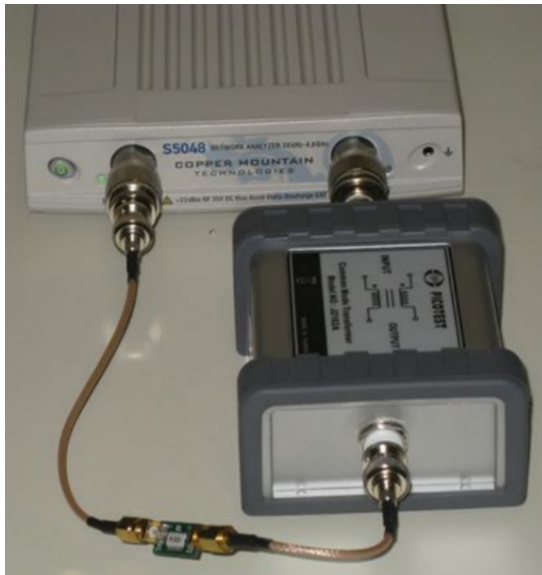
Figure 2: The 2-port setup with a 1mΩ resistor for measurement.
