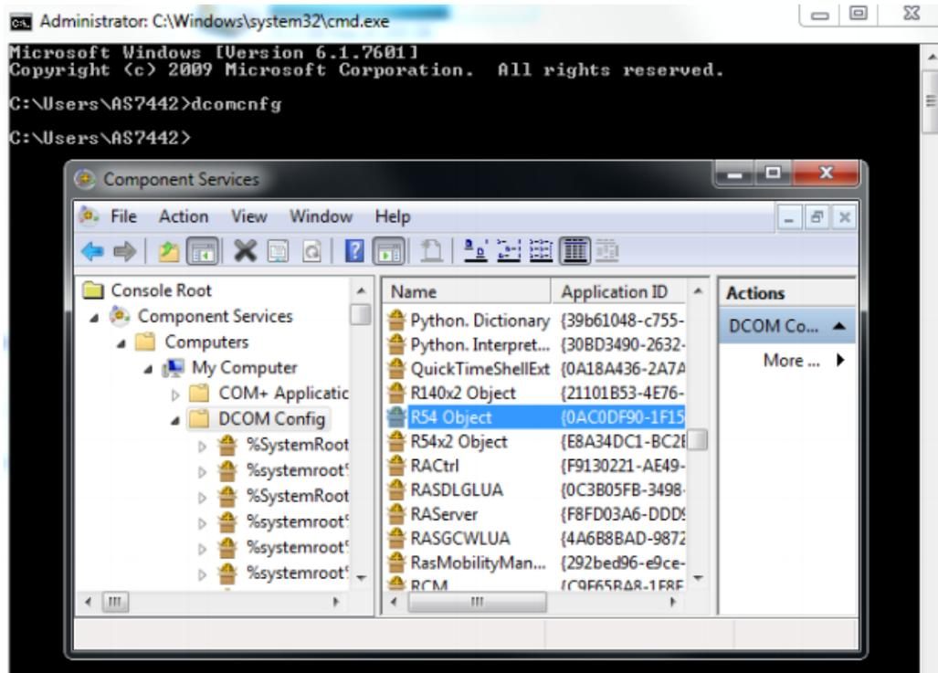
Figure 2: DCOM configuration of VNA application's object
