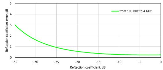
Specifications are based on isolating DUT ( $S_{21} = S_{12} = 0$ )
