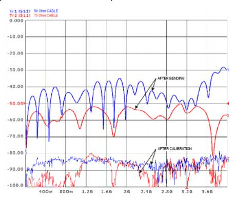
Using CMT Full-Size vector network analyzers with  $50\Omega$  test ports, 5.7 dB MLP connected to the VNA test ports, and performing SOLT calibration with a high-quality calibration kit, we can expect the measurement error to be dependent only on the quality of the calibration kit, keeping impact of the  $50\Omega$  to  $75\Omega$  adapter to a minimum.
