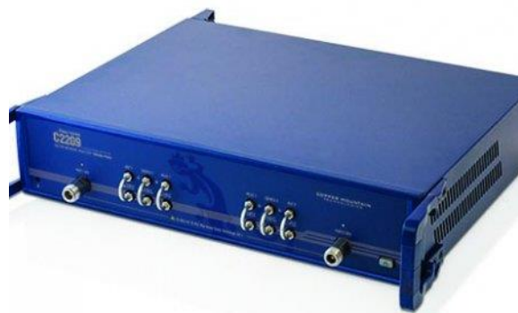
Figure 8 - Cobalt C2209, 9 GHz VNA with Direct Receiver Access
