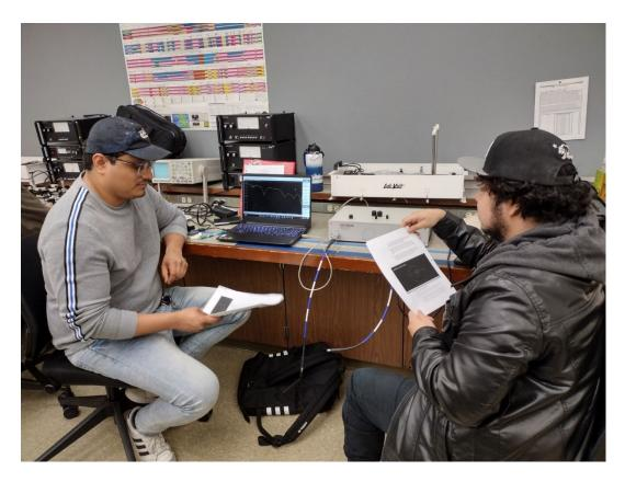
Professor Hymer has developed a lab curriculum to help teach VNA use to his students (<u>examples of the curriculum can be found here</u>). His labs provide context on the measurements involved, an overview of the DUTs, and details on calibration before a guided walkthrough of the measurement process. Once the students complete the lab, they answer questions about the measurements, DUTs, etc., and convey what they have learned.
