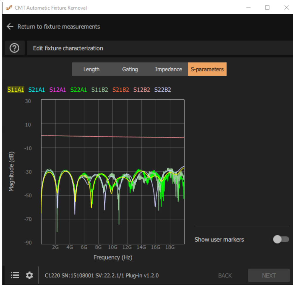
Figure 20 - Fixture Sides A and B S-Parameters
