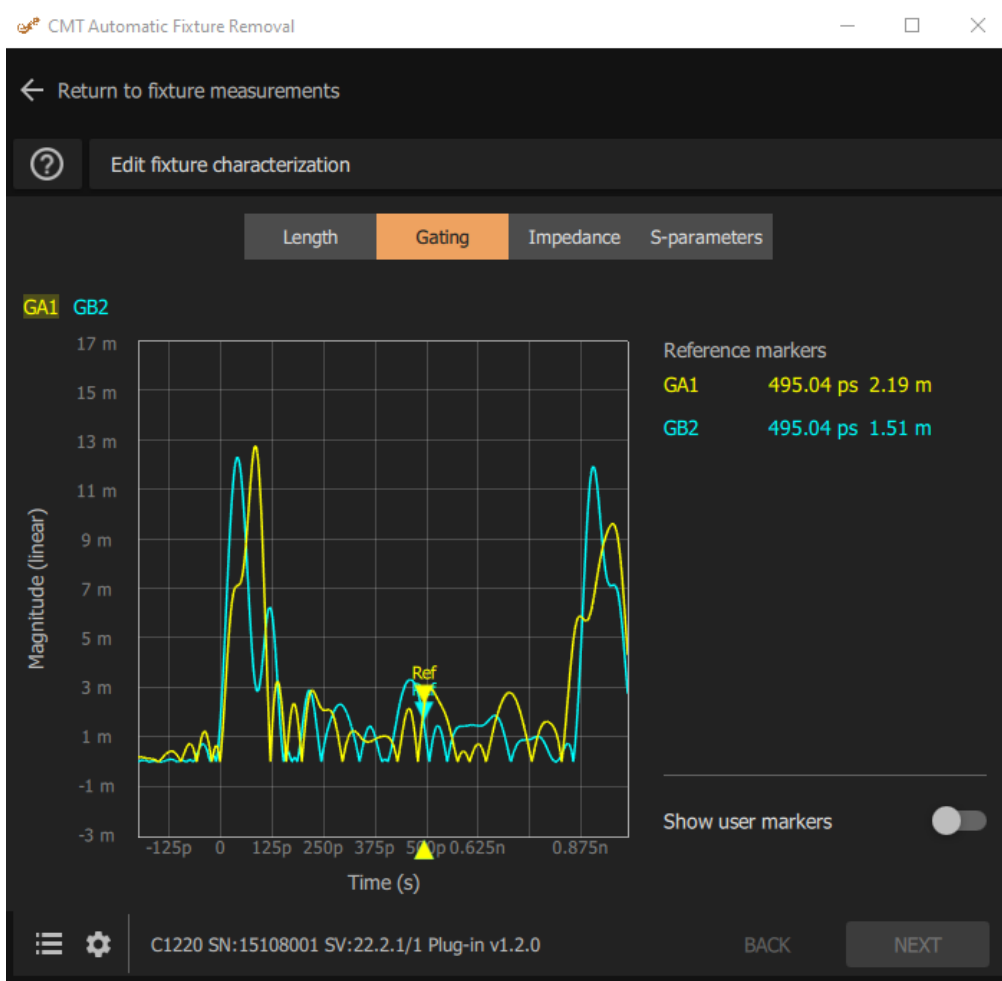
Figure 18 - Fixture Reflections in Time Domain
