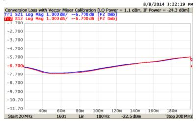
The RF and IF frequencies are swept while the LO was kept at 400 MHz. The upconverted signal was sent through a 420 MHz – 600 MHz (3 dB points) filter. This was coincidentally the range we chose for our measurements.
