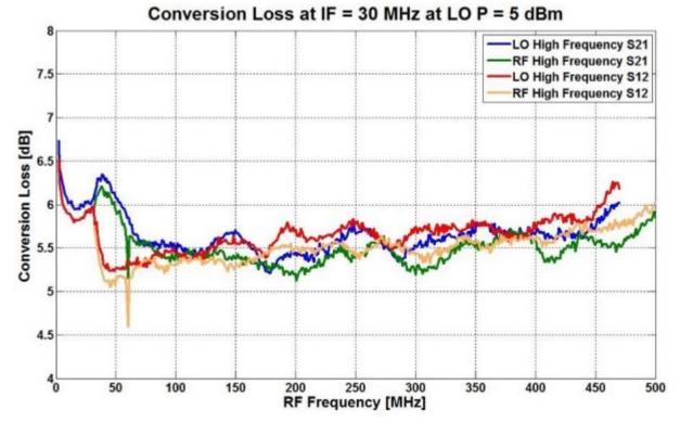
These conversion loss measurements were performed with the IF frequency fixed at 30 MHz and the RF Power at -25 dBm. The four measurements correspond to whether the LO or RF was the higher frequency and whether S12 or S21 was measured.
