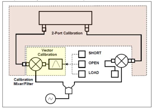
VMC is based on up- or down-converting a frequency to an intermediate level, sending the intermediate signal through a filter to remove spurious products, and then down- or up-converting the frequency back to its original level, so that frequency offset is not required and phase information can be measured by the VNA. In order to accurately measure the MUT, the calibration mixer and filter are de-embedded from the measurement.
