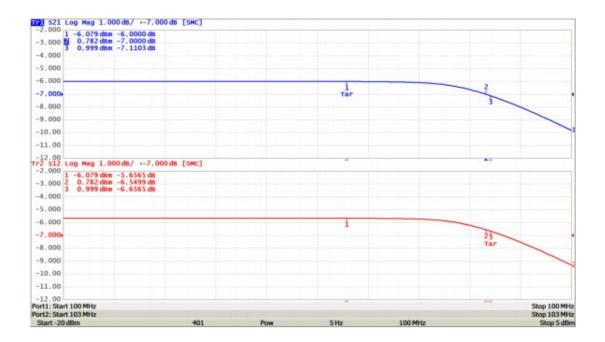
Here we performed a sweep of IF Power, with LO Power = 5 dBm and LO frequency = 3 MHz. The IF frequency is set to 100 MHz and the upper sideband RF signal is 103 MHz. The 1 dB point is approximately +0.75 dBm.
