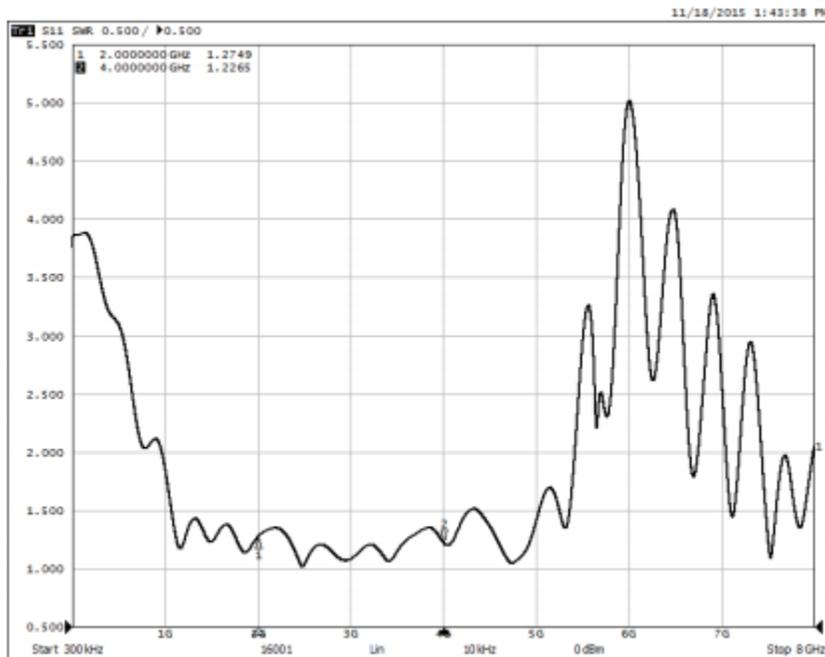
From the measurement results, we can see that the input VSWR, through the operating frequency, is always better than 1.4:1 and the transmission coefficient is about -6.4 dB for each output port. Therefore, our multiport testing system with RF switch is providing us a good measurement result that agrees with the datasheet.
