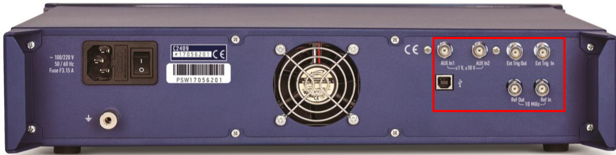
Figure 3: The rear panel of the C2409 also contains electrostatic discharge sensitive RF connectors
