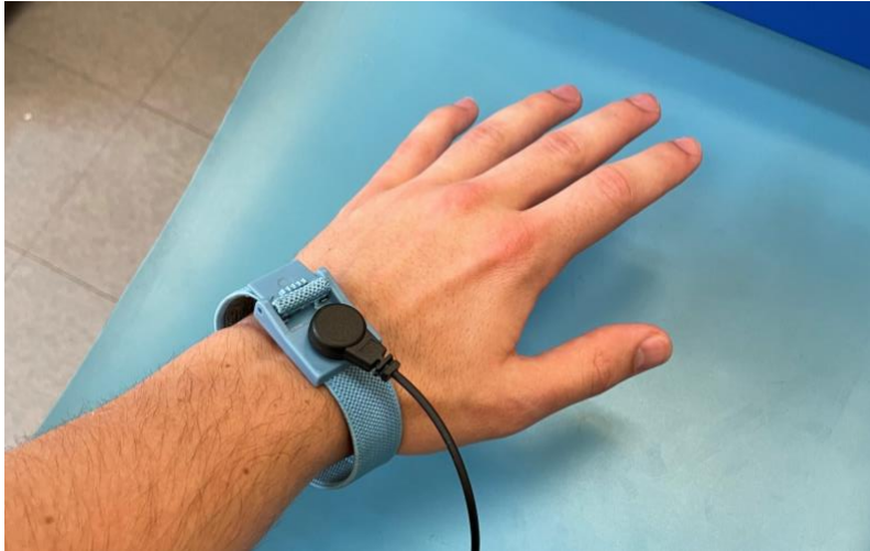
Figure 5: ESD grounding mat wrist strap
