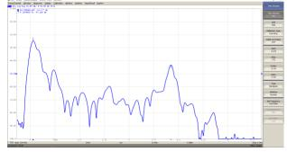
To use this function, choose the active trace and select *Analysis -> Time Domain -> Time Domain* to transform the trace. The horizontal axis will become nanoseconds and the data is now presented in time domain.
