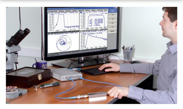
Our SC Series Compact VNAs deliver a small lab grade VNA with higher speed, more dynamic range, and higher output power, with all the features engineers have come to expect included: time domain and gating conversion, segmented frequency sweeps, linear/logarithmic sweeps, power sweeps, multiple trace formats, 16 channels max. with up to 16 traces each, marker math, and limit tests.
