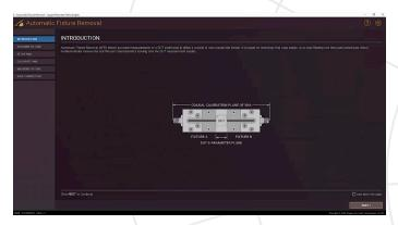
The Automatic Fixture Removal (AFR) plugin uses metrology grade de-embedding algorithms to eliminate fixture effects on your DUT. CMT offers 2xThrough fixture removal support with three methods that fit different fixture configurations:
